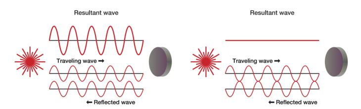
If the interference condition is fixed, it is easy to improve S/N. However, for example, due to changes in the emission wavelength of the laser or slight changes in the optical path length due to vibration or temperature change of the system, the interference conditions change over time and the improvement of S/N is not easy.
