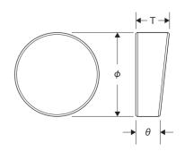
parallel window can be suppressed by using a wedged window instead. The wedged angle varies depending on the situation in which interference occurs, but it seems that in many cases, the effect is generally obtained at about 3 to 10 degrees.
