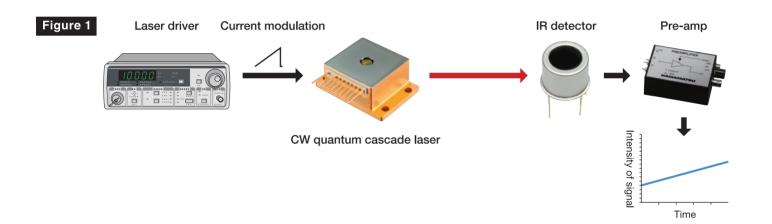
The forward current to the CW quantum cascade laser was increased at a constant rate and simultaneously emission wavenumber, i.e., wavelength was continuously scanned about 1 cm<sup>-1</sup> by means of current modulation. According to the current modulation, the signal intensity from the detector increased as the forward current of the CW quantum cascade laser increased.
