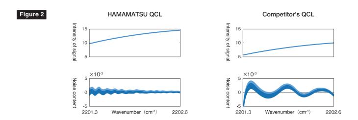
It can be seen that periodic fringe is observed as the emission wavenumber is scanned. The larger the amplitude of the fringe, the more the system S/N will be compromised. For comparison, the experimental results using another company's CW quantum cascade laser with built-in lens under the same experimental conditions are also shown. It is found that our lens built-in CW quantum cascade laser has lower fringe amplitude, resulting in lower optical noise.
